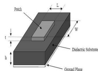
Fig.1. Structure of microstrip patch antenna
