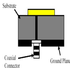
Figure:3 coaxial feed
