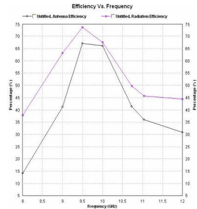
Figure 7 : Efficiency Vs frequency characteristics at 9.5 GHz
