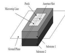
Figure 4 Rectangular Microstrip antenna Aperture coupled feed
