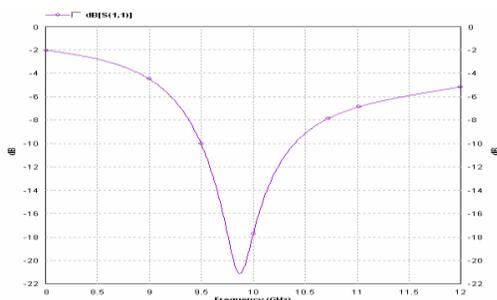
Figure 6 Simulated return loss characteristics at 9.5 GHz
