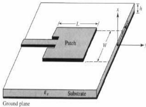
Figure 2: Microstrip antenna
