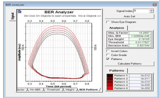
Figure.6: Graph Showing bit error rate using Erbium Doped Fiber Amplifiers for dispersion
