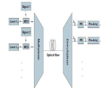
Fig. 2: Schematic diagram of a point-to-point WDM link
