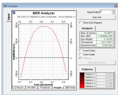
Fig 5: Graph Showing Signal height using Erbium Doped Fiber Amplifiers for dispersion compensation
