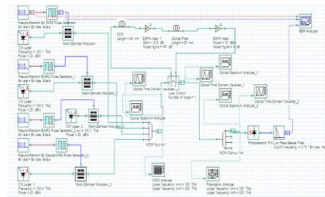
Fig. 3: Dispersion compensation using Pre DCF
