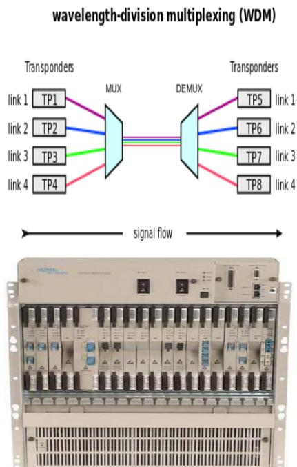
Fig. 1 Wavelength division multiplexing
