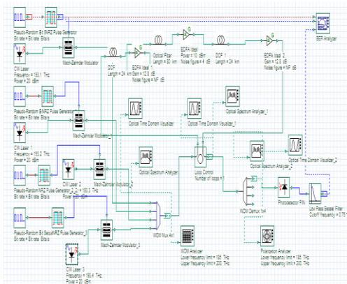
Fig. 4: Dispersion compensation using Symmetrical DCF
