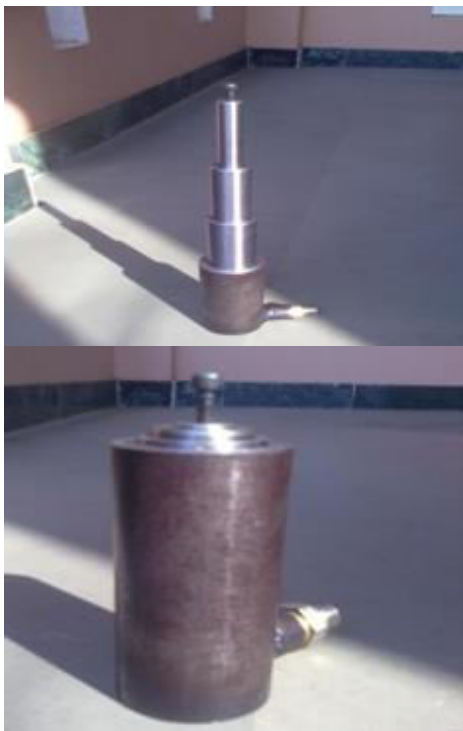
Fig.13. Fabricated hydraulic Actuator
