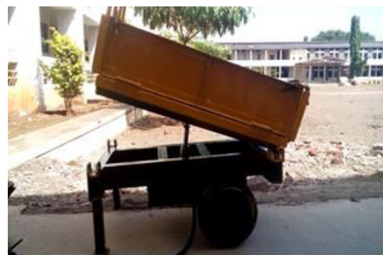
Fig.16. Fabricated trolley- Back dumping
