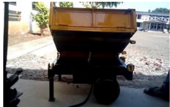
Fig.15. Fabricated trolley- Right side dumping
