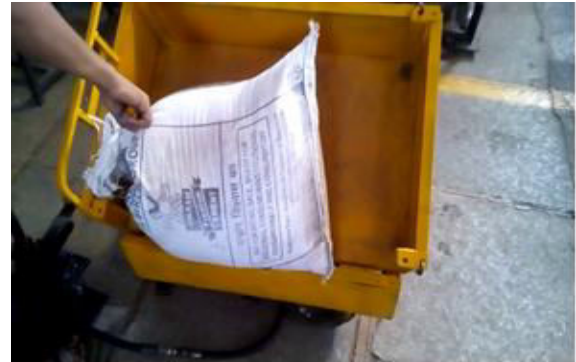
Fig.14. Fabricated trolley- Left side dumping
