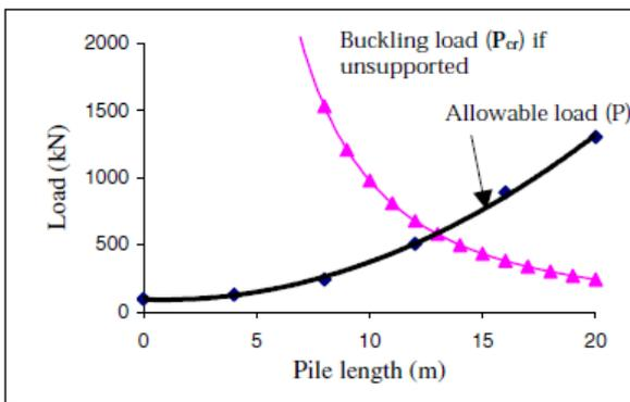
**Fig.7:-Allowable Load And Buckling Load Of A Pile (If Unsupported)**
