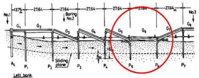
**Fig.6:-Schematic Diagram Of The Failure Of The Showa Bridge.**
