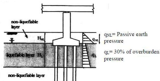
**Fig.2:- Schematic Sketch Showing Pressure Distribution against the Piles due to Lateral Soil Flow associated with Liquefaction (JRA, 1996)**
