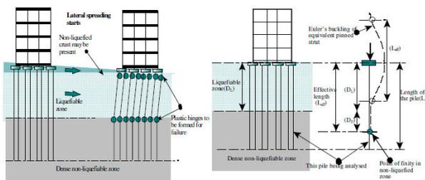
**Fig.8 (A): Combined mechanism of axial and bending.**
