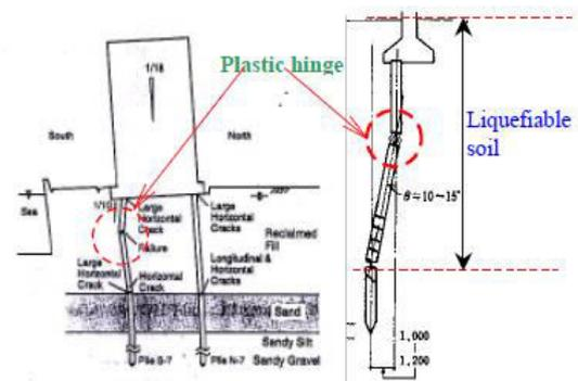
**Fig.4:- Collapsed buildings showings location of plastic hinge**
