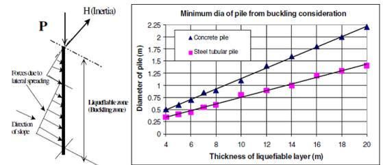
**Fig.9 (A): Free body diagram\_\_\_\_\_ Fig.9 (B): Chart connecting diameter of pile and showing the generalized loading thickness of liquefying layer acting on a pile.**
