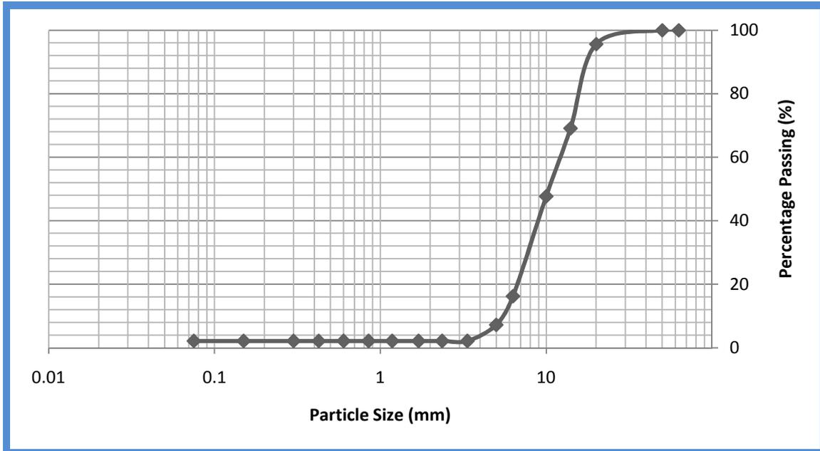
Fig.2: particle size analysis of the coarse aggregate
