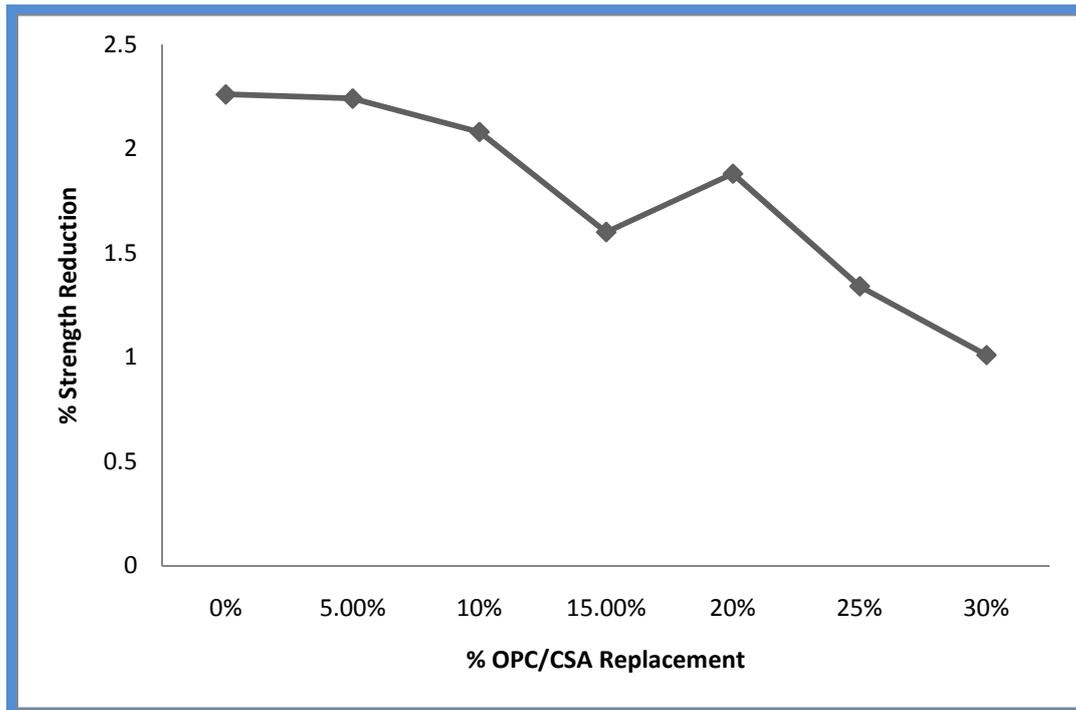
Fig.6: Percentage reduction in the compressive strength of OPC/CSA concrete in sulphate solution curing medium
