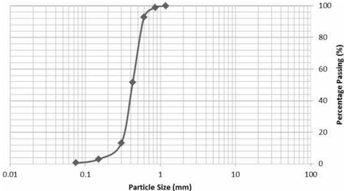
Fig.3: particles size analysis of coconut shell ash
